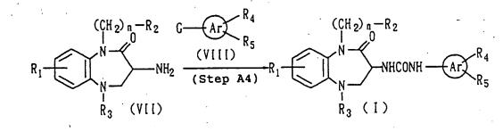
(wherein A represents a tert-butoxycarbonyl group or a benzyloxycarbonyl group; B represents a halogen atom; E represents a halogen atom; G represents an amino group, an isocyanato group, or a carboxyl group; and R1, R2, R3, R4, R<sub>5</sub>, Ar, and n represent the same as defined above).
